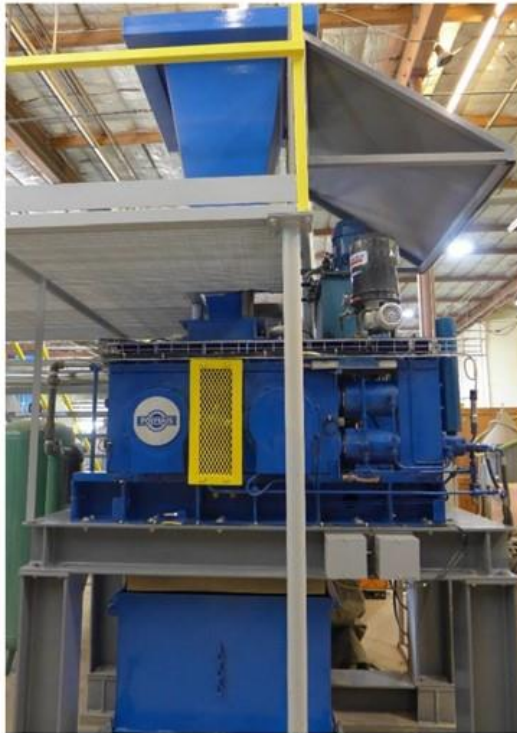
Figure 13-11. View of SMALLWAL HPGR unit at KCA Used for Testing Hasbrouck Mine Samples
